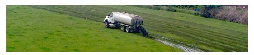
Part of the wastewater treatment process is the treatment and processing of biological solids from the water. Each year, Troutdale's Water Pollution Control Facility produces more than 3 million gallons of digested sludge in its lagoon. This results in nutrient-rich organic materials called biosolids. In the past, biosolids were viewed as waste and disposal options included landfill or burial, incineration, and dumping at sea. Now there is a much better option.
